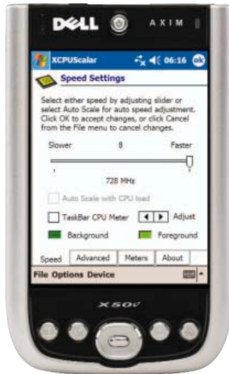
XCPU Scaler unlocks the dynamic scaling capabilities of Xscale processors used in modern PocketPC PDAs, allowing you to over or underclock them. Here the 624MHz processor of a Dell X50v is being overclocked to 728MHz
